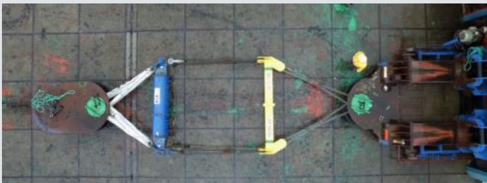
Figure 4: Tension test of a 150 MT spreader beam
