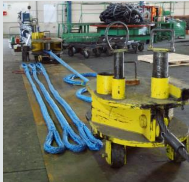
Figure 2: Pre-stretching and measuring synthetic slings
