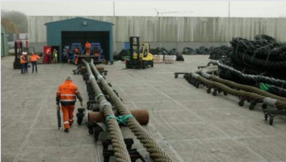
Figure 3: Cable-laid grommet length measurement under tension
